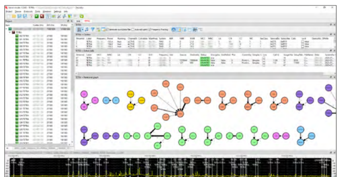
Automatic TETRA decoding and metadata display
