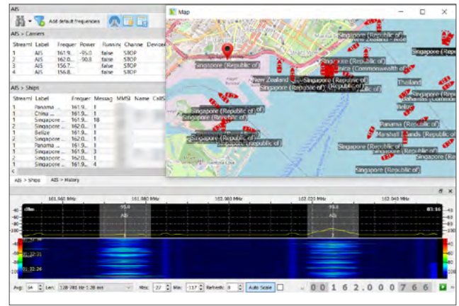
Easily display and save record air and maritime transmissions, including positions (ADS-B, ACARS, VDL2, FLARM, AIS)
